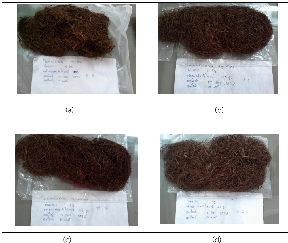
Figure 3 Green coconut fibers extracted by steam explosion method (a) 17 Bar at 207 °C for 5 minutes (b) 17 Bar at 207 °C for 10 minutes (c) 18 Bar at 209 °C for 5 minutes (d) 18 Bar at 209 °C for 10 minutes
